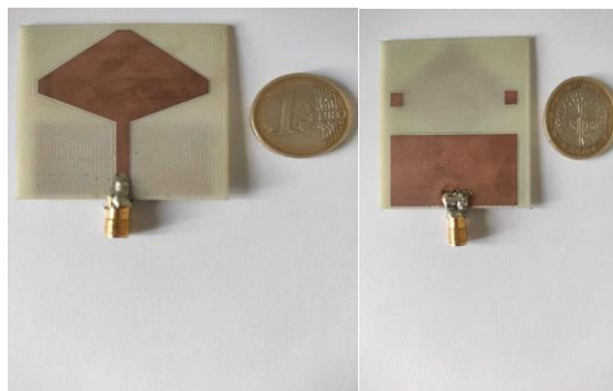
Fig. 10. Prototype of the proposed antenna.
